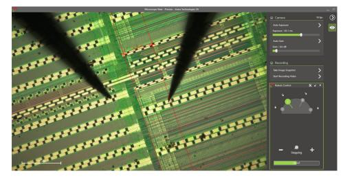
Precisio<sup>™</sup> software microscopewindow with controls for imaging parameters, tools for recording, annotation, and dimensional measuring.
